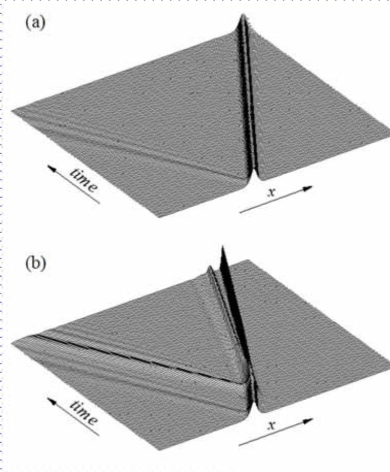
Wave profiles for a solitary wave propagates over a step
