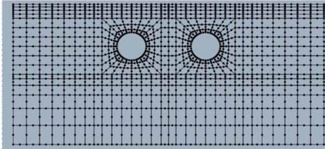
Mesh for two circular cylinders (8-node quadrilateral element)
