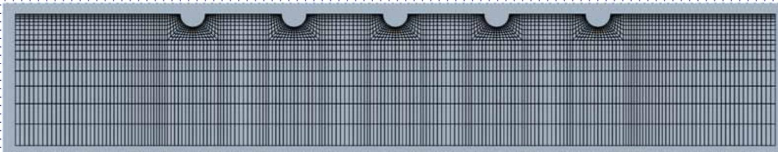
Mesh for five floating semicircular cylinders (8-node quadrilateral element)
