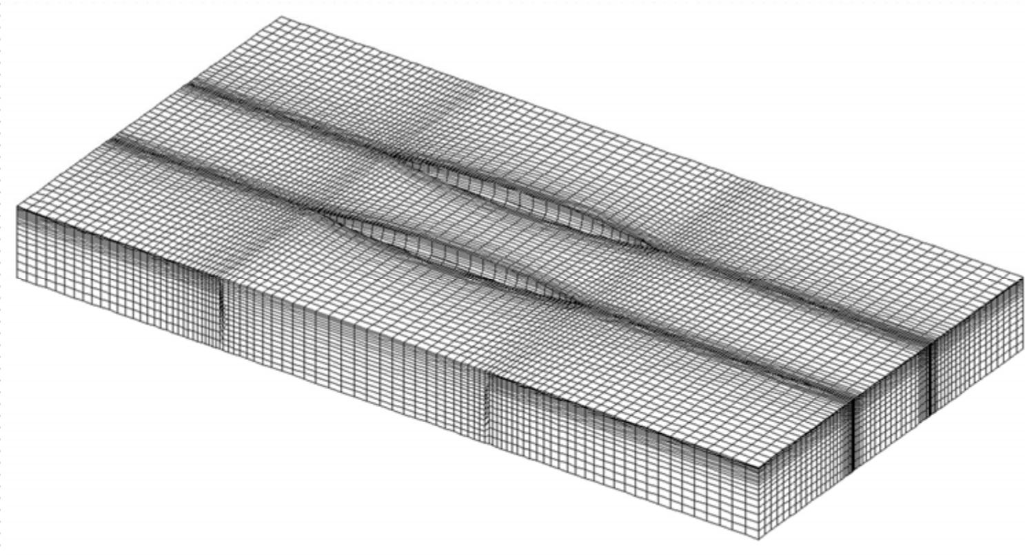
3D mesh for a twin Wigley ship (20-node brick element)
