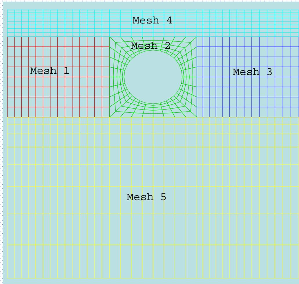
A multi-block mesh for a circular cylinder formed by combining five simple meshes together
