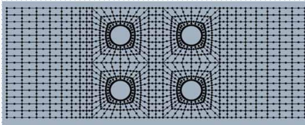
Mesh for four circular cylinders (8-node quadrilateral element)
