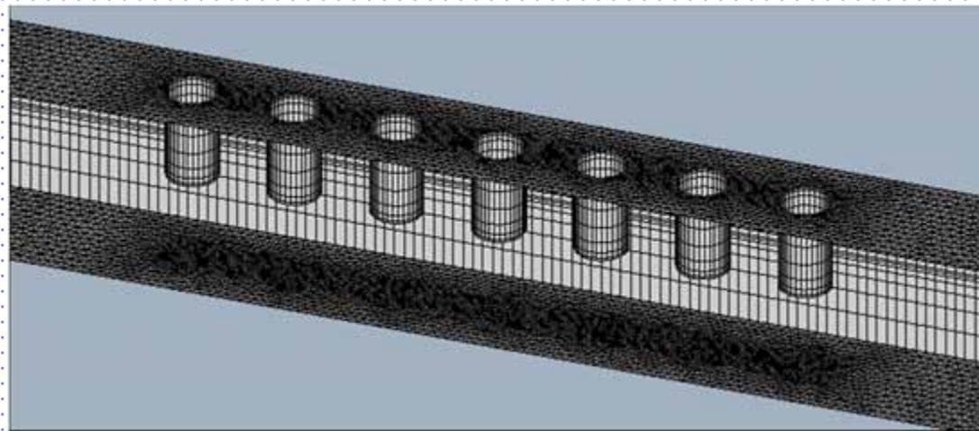
Seven truncated cylinders (6-node prism element)
