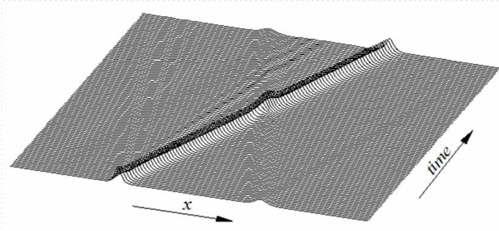
Wave profiles for two waves colliding with each other
