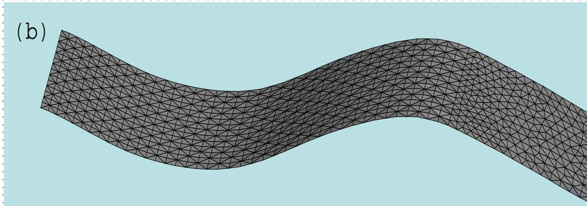
(a) Unstructured mesh without smoothing; (b) Hybrid mesh with smoothing applied within structured mesh (Wu, Ma & Eatcok Taylor 1996, 21st ONR, Trondheim)
