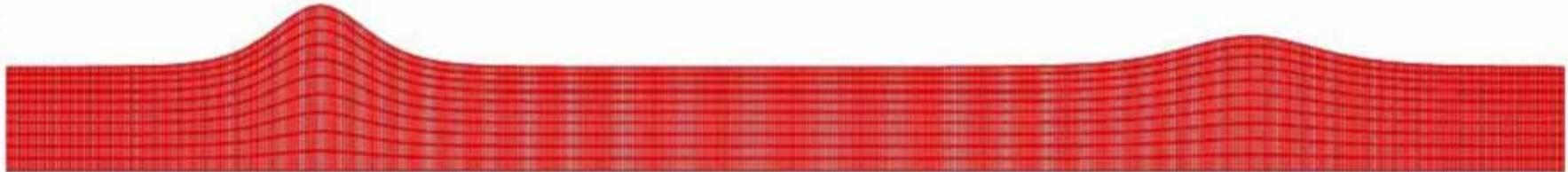
Finite element mesh for two solitary waves colliding with each other (8-node quadrilateral element)
