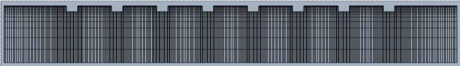
Mesh for eight floating rectangular cylinders (8-node quadrilateral element)
