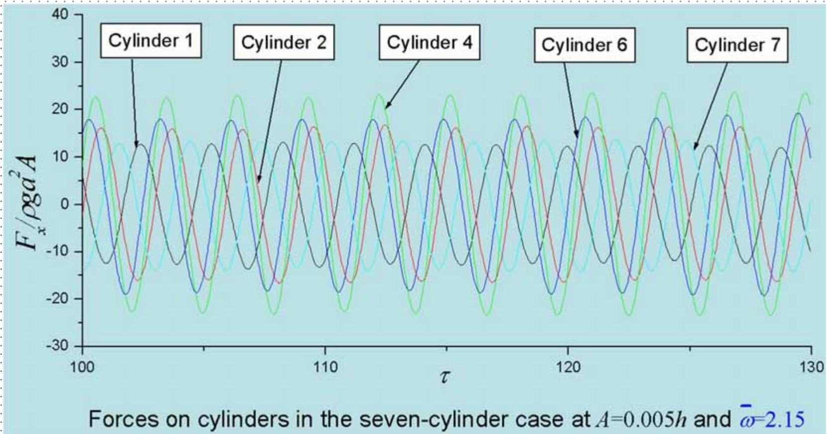
The maximum force is on the middle cylinder (cylinder 4)
