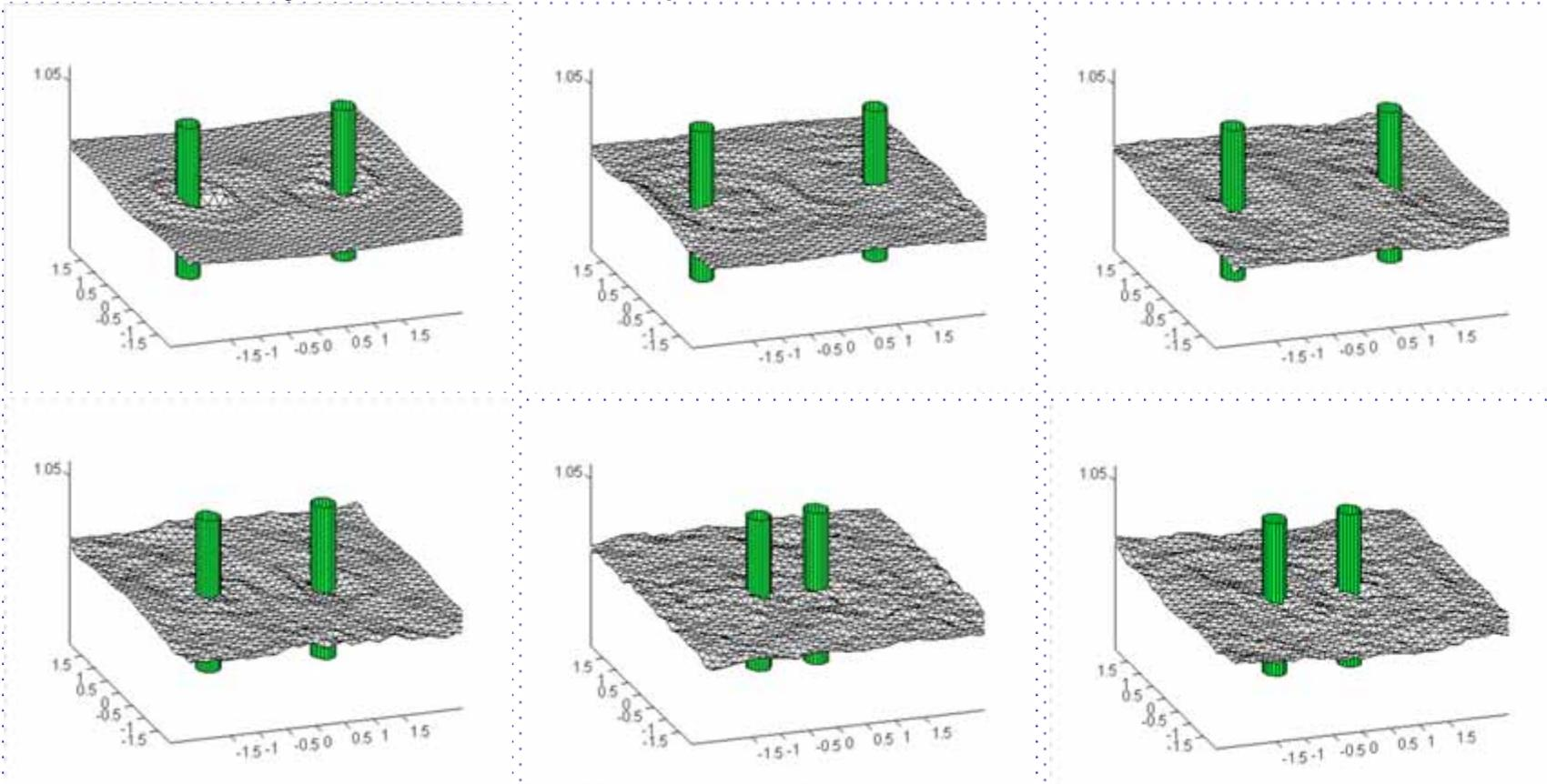
Wave profiles by two cylinders undergoing periodic oscillation
